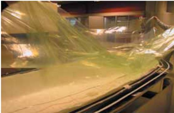
Foil types that have shown to work the best are nylon based. The foil should be wide enough to cover the whole part. Splicing of foils should be avoided, as this can often cause vacuum leakage.
